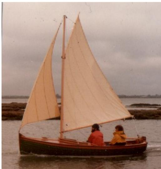
This dinghy has similarities with North American yawl boats and some Scottish craft, being a developed rowing boat form – thus she has fine lines below the waterline and slack bilges to give an easily driven hull. Above the waterline the topsides flare to a wide beam with good freeboard to make a dry sailing hull with good reserve stability and plenty of space for the crew, with space for up to four adults.
